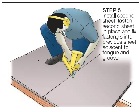
FIGURE 6 FIXING 2ND SHEET
