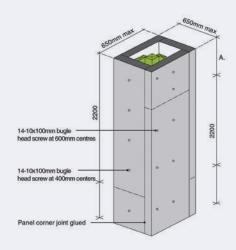
NOTE: THIS DETAIL IS NOT SUITABLE FOR SUSPENDED PANELS
