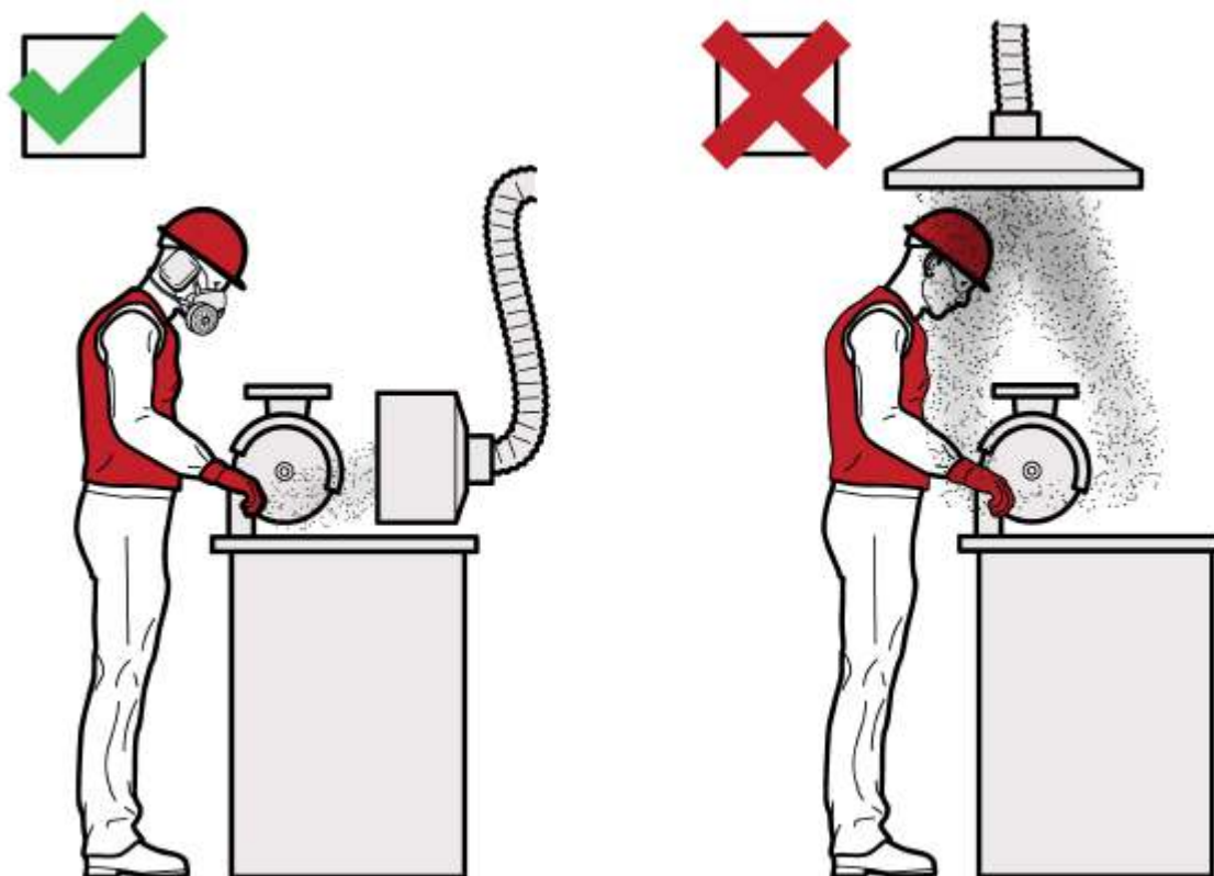
Figure 7 Examples of using local exhaust ventilation
