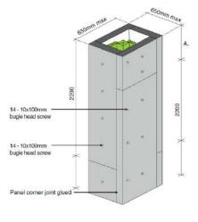
NOTE: THIS DETAIL IS NOT SUITABLE FOR SUSPENDED PANELS MAXIMUM SQUARE COLUMN SIZE 650MM X 650MM MAXIMUM RECTANGULAR COLUMN SIZE 700MM X 600MM 'A' DENOTES STAGGERED PANEL JOINT
