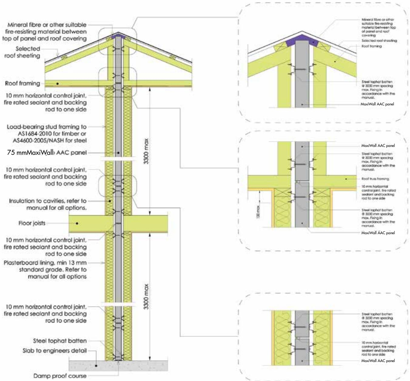
\* To achieve discontinuous construction for acoustic requirement under the NCC, the horizontal panel must be installed on top of the vertical panels for each floor level.
