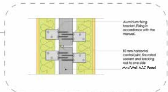
\* To achieve discontinuous construction for acoustic requirement under the NCC, the horizontal panel must be installed on top of the vertical panels for each floor level.
