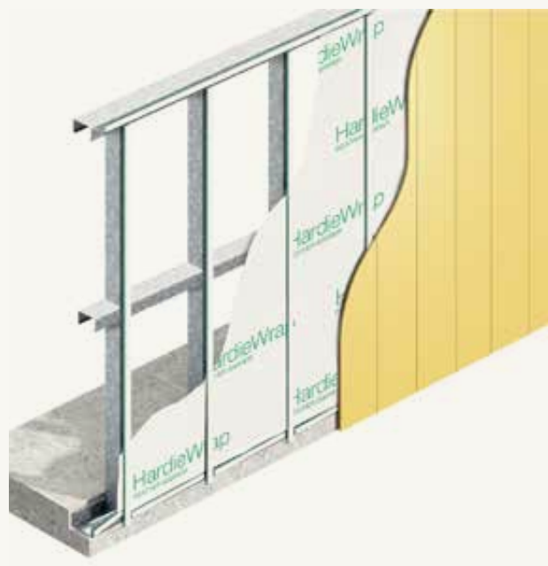
Installation of HardieBreak™ thermal strip for flat sheet direct fix
